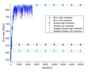
Fig. 6: Grid effect. In the legend, "low resolution" describes a grid with 10 meters granularity, whereas, "high resolution" corresponds to a 5 meters 3D grid step granularity. A setup of 5 UAVs and 45 users in  $450m \times 450m$  is considered.
