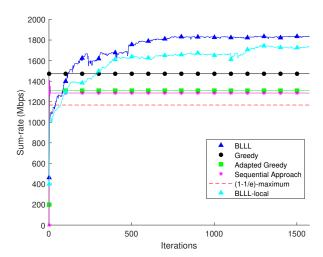
Fig. 5: Sum-rate convergence of BLLL, greedy, adapted greedy, and BLLL-local algorithms, and a suboptimal approach that solves the problem sequentially. Here,  $\theta=82.5$  dBm for BLLL-local algorithm.
