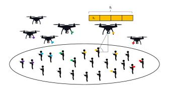
Fig. 1: The figure shows the setup of our problem. UAVs have designated bandwidths  $B_j$  divided into subchannels  $b_j$  that they can assign to different users. Users assigned to UAVs are indicated by circles of the same color as the UAV.
