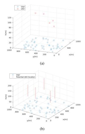
Fig. 2: (a) Initial configuration (b) Potential locations of UAVs using k-means.
