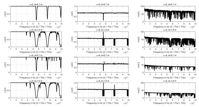
Fig. 4: Estimated channel parameters  $\hat{\psi}(d, f)$ ,  $\hat{\sigma}(d, f)$ , and  $\hat{m}(d, f)$  with different spreading loss exponents and transmission distances, given S = 1000,  $\zeta(d, f) = 1$  and  $\eta(d, f) = 1$ .
