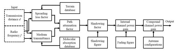
Fig. 1: Holistic procedure of compound channel modeling, integrating spreading loss, molecular absorption loss, shadowing, multi-path fading, and antenna configurations.
