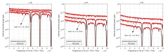
Fig. 3: Internal channel power gain versus radio frequency for cases with different transmission distances, given  $\zeta(d,f)=1$  and  $\eta(d,f)=1$ .
