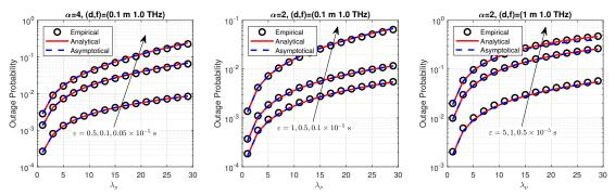
Fig. 6: Outage probability versus outage threshold with average packet arrival rate with different outage threshold, given L=10 bits,  $\zeta(d,f)=1$ , and  $\eta(d,f)=1$ .
