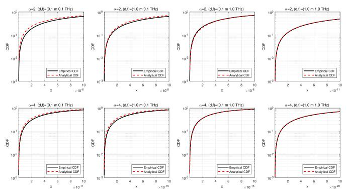
Fig. 5: Comparison between the empirical and analytical CDFs of the internal channel power gain, given  $\zeta(d, f) = 1$  and  $\eta(d, f) = 1$  (the x-axis scales of subplots are varied so that the key distribution regions can be clearly shown).
