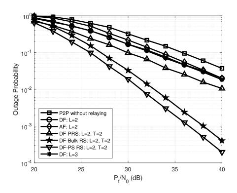
**Figure 5.** Outage probability comparison among point-to-point plain OFDM-IM system and various relay assisted OFDM-IM systems with different system configurations.
