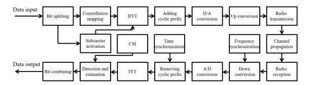
Figure 1. System diagram of a typical DF relay assisted OFDM-IM system.
