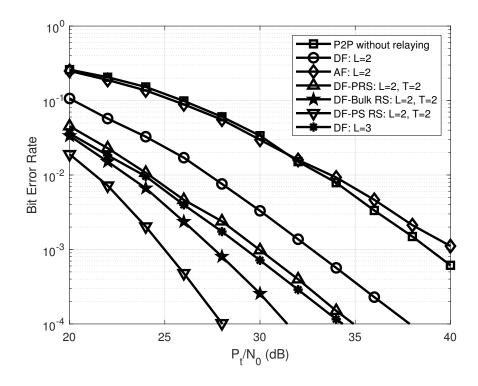
**Figure 4.** BER comparison among point-to-point plain OFDM-IM system and various relay assisted OFDM-IM systems with different system configurations.
