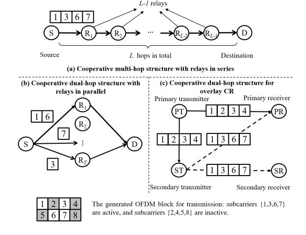
Figure 2. Three major cooperative multi-hop structures for relay assisted OFDM-IM.
