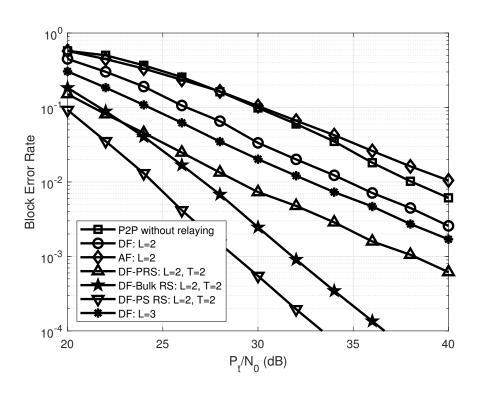
**Figure 3.** BLER comparison among point-to-point plain OFDM-IM system and various relay assisted OFDM-IM systems with different system configurations.
