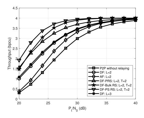
**Figure 6.** Throughput comparison among point-to-point plain OFDM-IM system and various relay assisted OFDM-IM systems with different system configurations.
